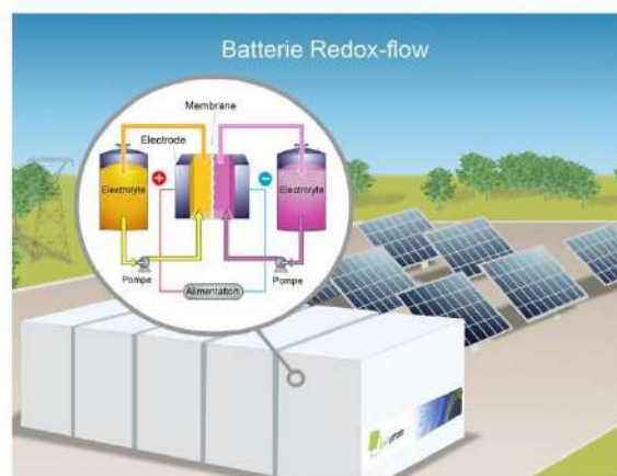
Figure 35 : Principe des batteries redox-flow Source CEA
